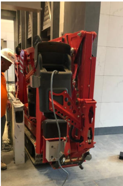
Minimum pass-through width of 0,78 m due to the removable platform
