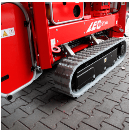
Hydraulically height- and width adjustable crawler tracks for driving on slopes
